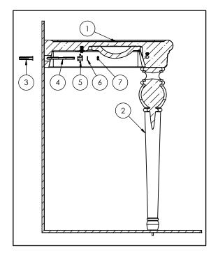
4. Place rawlplugs (3) in previously drilled holes. Again, place basin (1) on legs (2). Screw hanger bolts (4) into rawlplugs (3). Fix the basin to the wall using plastic cover (5), washers (6) and nuts (7).
