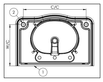
1. Check measurements from centre to centre of each leg (C/C) and from centre of leg to the wall (W/C). Compare these to the guide on page 1.
