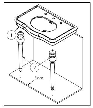
2. Drill holes in floor in accordance with the previously taken measurements. Embed legs (2) in the drilled holes. Place basin (1) on legs (2). The basin has to be held up constantly (preferably by two people) during this operation. While the basin is being held up, another person can install it.
