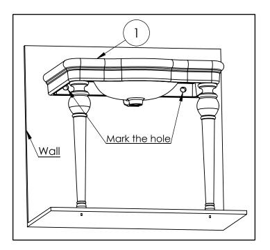
3. Level basin (1) and mark the holes on wall from underneath of the basin. Remove the basin and drill the holes.
