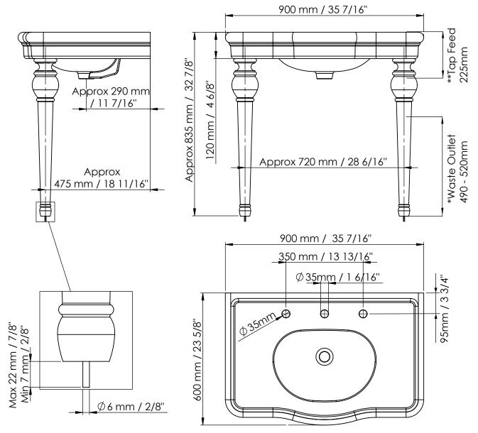
\* Guide height using a Drummonds Waste and Bottle Trap. \*\* Recommended height using Drummonds' taps and pipework set. This measurement can be changed to suit your installation.
