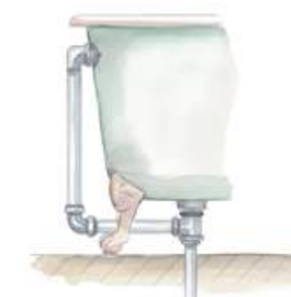
Above the floor waste
